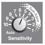
It is always recommended to adjust the manual sensitivity as high as possible without producing false signals. For example, turn the control anticlockwise until false signals are heard, then slowly adjust clockwise until the false signals 'just' stop. Setting the Excalibur II so that it is 'just' stable, will ensure maximum depth and sensitivity whilst still hearing faint signals. Set too high and increased noise may mask faint signals. Set too low and the detector may not hear faint signals.
