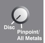
The Excalibur II can operate in two different modes. This control selects either Disc (Discriminate) or Pinpoint/All Metals mode.
